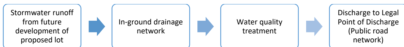
Figure 4: Proposed Water Quality Treatment Train
